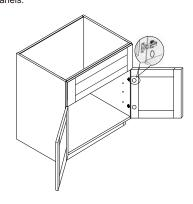
**Step 6:** Adjust the hinges to ensure that the clearance for all doors is the same. Finally, check the firmness and stability of the cabinet tightening the cam locks as necessary.
