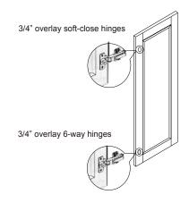
**Step 5:** Connect the doors to the box, hinges on the door panels snap into the hinges on the side
