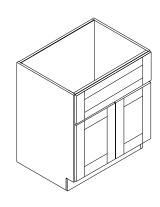
**Step 2:** Assemble the cabinet using cam locks and wood dowels. Start by screwing in all the male ends of the cam locks and inserting the wooden dowels. When the sides, bottom base and braces are loosely connected, tighten everything with the female part of the cam locks. Finish by sliding the back panels into its groove.
