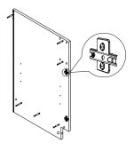
**Step 3:** Install the front panel to the front brace and attach using screws.
